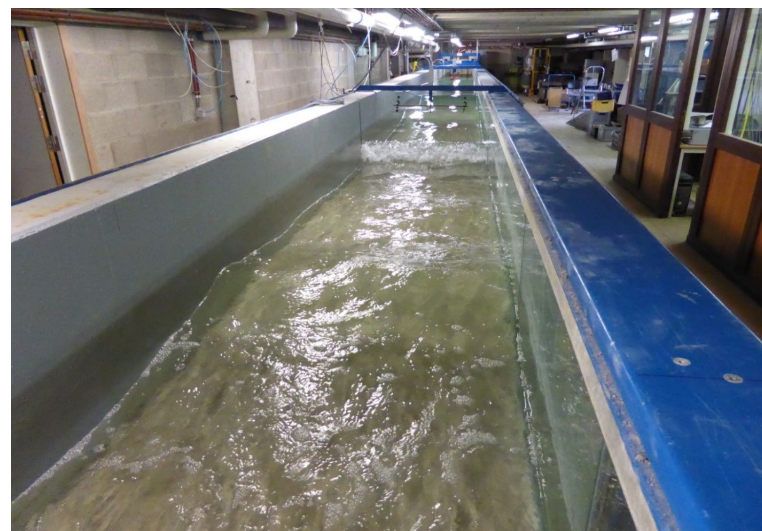
Hydraulic modelling using the 30 m long wave flume facility at Ghent University
